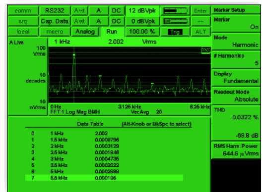
Use the SR785 to monitor the fundamental and harmonics of your signal. Total harmonic power and THD are calculated in real-time for fast, accurate analysis.
