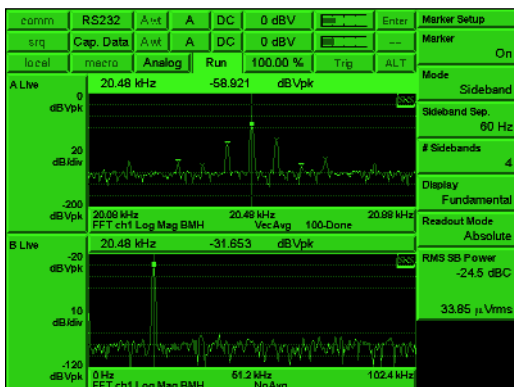
Bottom display shows a wideband FFT, while the top display shows a narrowband FFT of the same signal. The sideband marker has been selected for calculation of the total sideband power.
